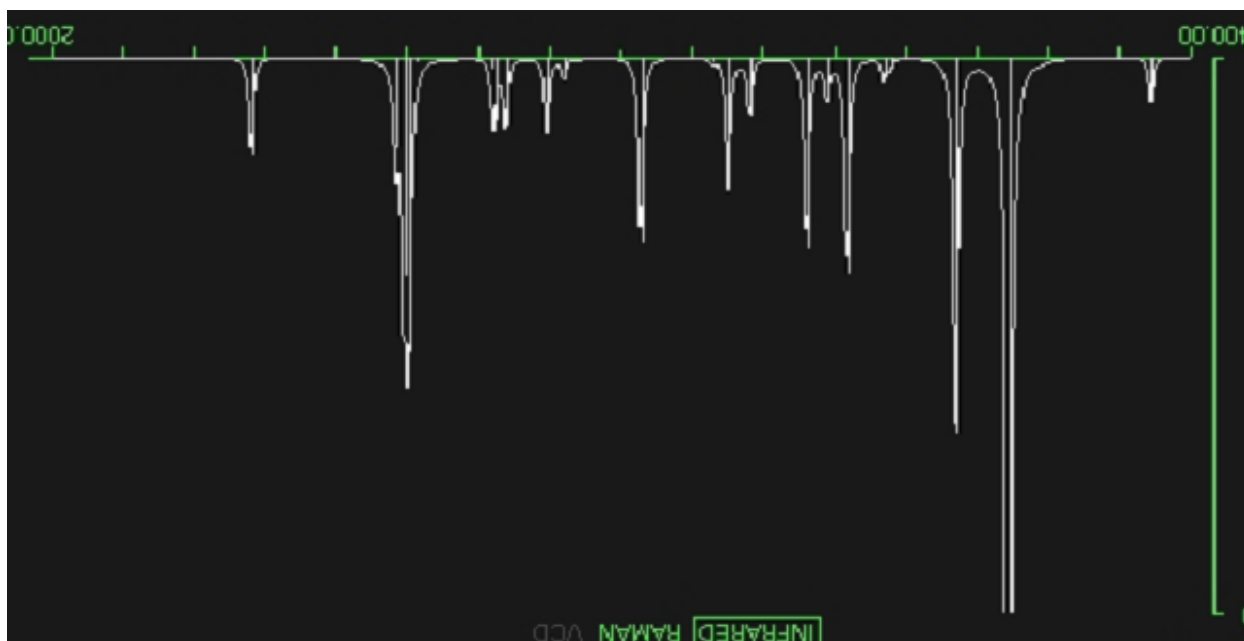
Cyclohexene calculated IR spectrum (unscaled)
